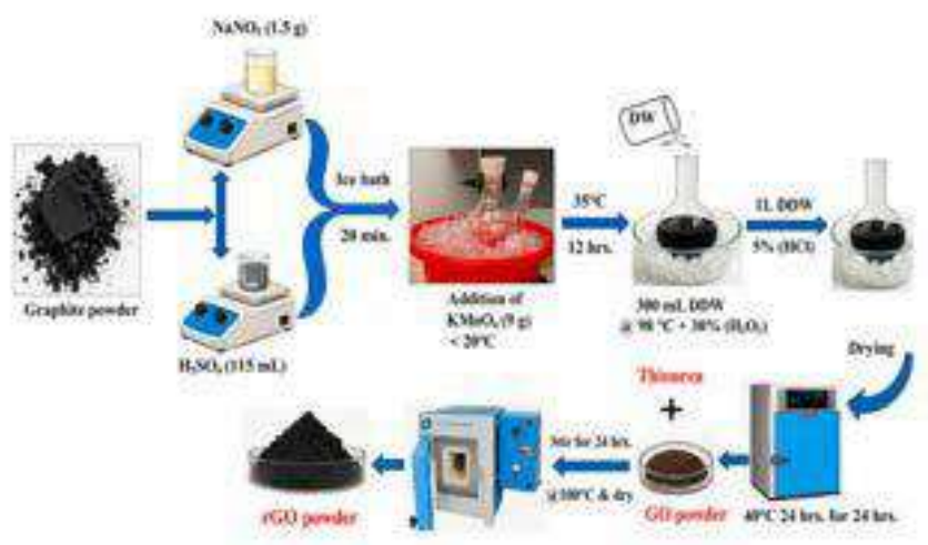
Figure 1. Schematic depiction of GO and rGO synthesis using modified Hummer's Method
