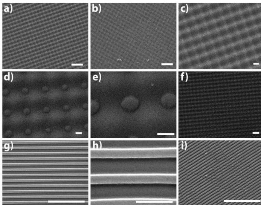
**Figure 1:** A, D, G) SEM image of the diffraction grating template, diffraction glasses and DVD respectively. B, E, H) Replications of the templates A, D, G fabricated in PDMS and C, F, I) fabricated in PLA. Intro scale bars A, B, F) 10  $\mu\text{m}$ ; C) 5  $\mu\text{m}$ ; D, E, G, H, I) 1  $\mu\text{m}$ .
